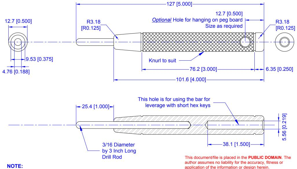
3/16 inch diameter is the size used for the Taig 3 soft jaw scroll chuck.
